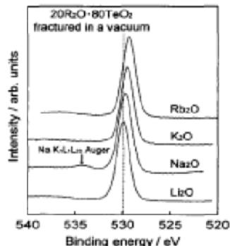
Fig. 3. O 1s photoelectron spectra for  $20\text{Rb}_2\text{O}\cdot 80\text{TeO}_2$  (R: Li, Na, K and Rb) glasses.
