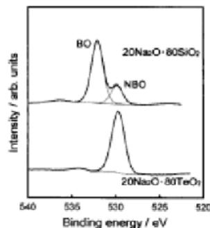
Fig. 7. O 1s photoelectron spectra for  $20\text{Na}_2\text{O} \cdot 80\text{TeO}_2$  and  $20\text{Na}_2\text{O} \cdot 80\text{SiO}_2$  [21] glass. Solid lines and dotted lines represent the experimental spectra and resolved Gaussian-Lorentzian components, respectively.
