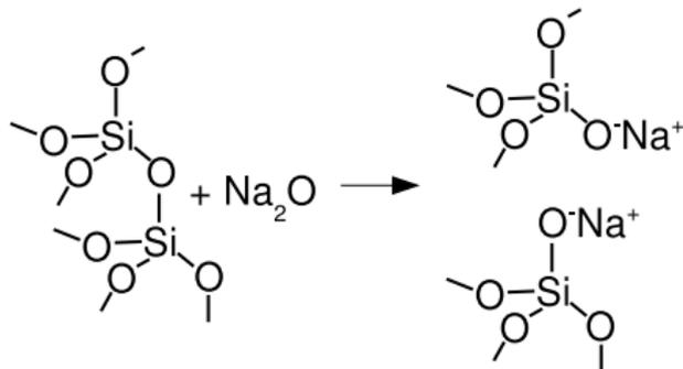
The nonbridging oxygen bonds are shorter than the original bridging oxygen.
