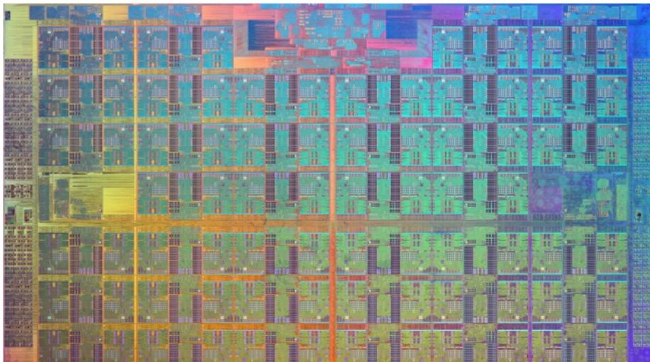
Intel Many Integrated Cores (MIC) Xeon Phi
